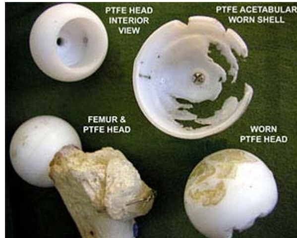
Figure 1.1: Sir John Charnley's early hip replacement designs made from PTFE showing very severe wear.[1]
