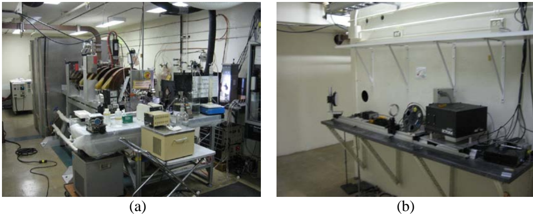
Figure 2.3: Photographs of the 6 MeV LINAC at the Notre Dame Radiation Laboratory. The LINAC (a) and monochromator and photomultiplier (b) used in pulse radiolysis experiments detailed in sections 2.6 and 4.2.
